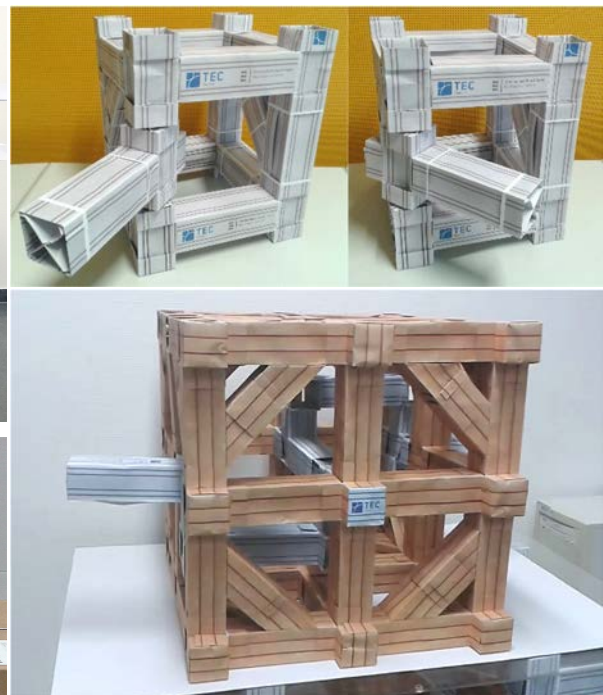
Figure 4: top: compliant pivot joint with 180° free motion range; bottom: kinematic linkage demonstrator, folded from 320 A4 sheets
