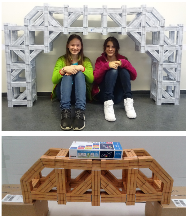
Figure 3: Truss bridges; top: 2 m wide, folded from 700 A4 sheets; bottom: 90 cm wide, 150 A4 sheets, carrying a pack of printer paper (3.1 kg)
